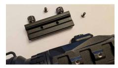
3. Clean any debris or residue off both the surfaces that seat against each other on the riflescope and mount.
