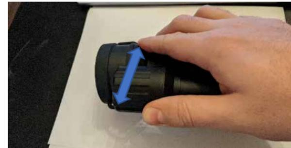
3. Twist the front of the IR to adjust focus, for longer range you will need to focus the beam to a smaller size.
