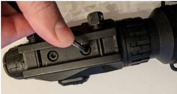
5. Reattach the mount to the firearm applying even pressure to both bolts.
