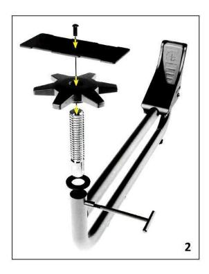
Next, screw the cradle plate to the top of the ram using the button head screw. There is a locating tab on the bottom of the cradle plate that matches the slot cut into the ram. When they are correctly aligned, firmly tighten the screw.
